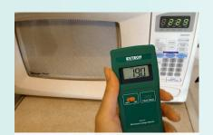
Easy-to-use, compact microwave leakage detector designed to measure high frequency radiation levels emitted from household and commercial microwave ovens.
